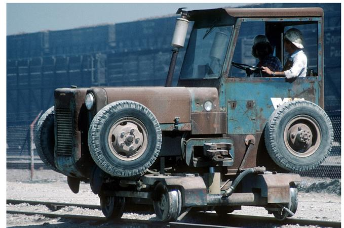
One of these scanned photos is shown above. This is a piece of switching equipment that could run on road or rail. In this configuration it ran on the rails and was ready to switch (note the coupler between the two large rubber tires).
