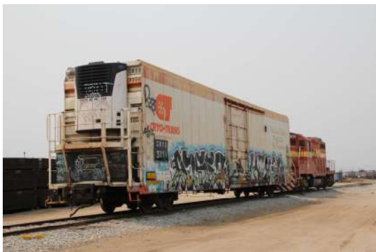
GPS Monitored 64 foot Jumbo Reefer in Osburn Yard
