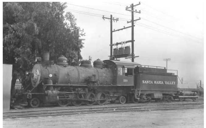
SMVRR #150 in the yard with its boiler jacket removed
